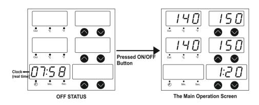
The cooked product is placed into the oven. When the device is energized, it is opened in off status and DISB clock appears. The on/off button is pressed to turns the main operation screen. The set values are values that existed before the device turns off. 📝 The temperature start button is pressed to start cooking. Set values can be changed while cooking. temperature stop button is pressed to stop cooking.
